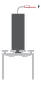
**5.** Bend the power connector (E) so that it fits into the sleeve (B). Put an arm with thread through the connector and secure it with nuts (D, G) and a locking washer (F).
