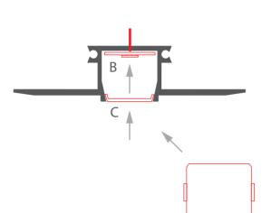
**2.** Attach the fixture (A) to the ceiling surface and connect the power cable.
