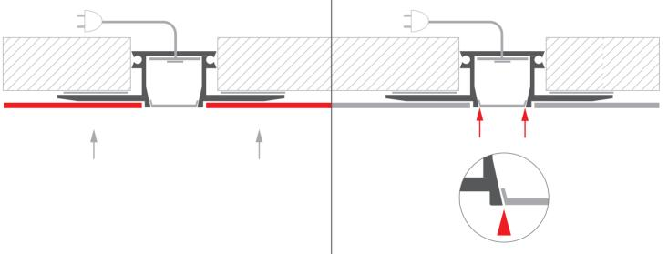
**5.** Remove the technical cover (C) and then insert the proper cover (D).
