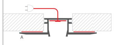
**3.** Apply a layer of plaster to the extrusion and the ceiling and then paint the surface.
